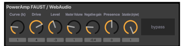
Fig. 13: GUI generated by the FAUST IDE, some extra parameters (negative feedback gain, waveshaper; drive, curve, saturation) are tweakable, enabling fine tuning of the NFB loop.
